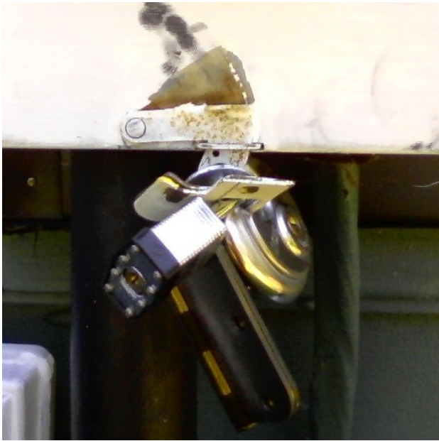
Pic 3. Box with shielded shackle lock thru loop and additional locks and hardware attached thru the lock's loop.
